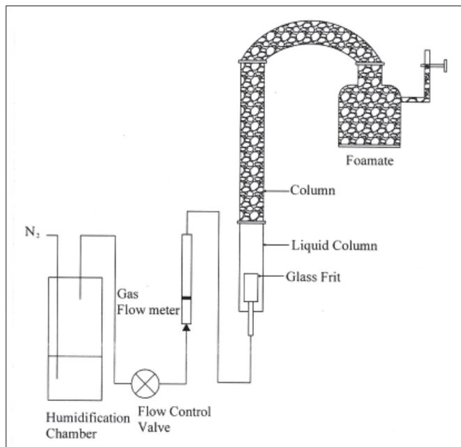
FIGURE 1. Schematic diagram of foam fractionation apparatus.
