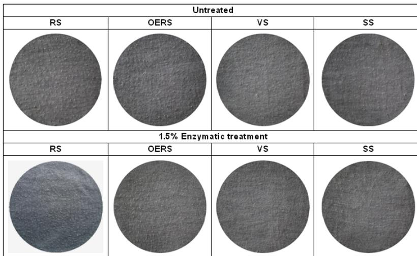
**Figure 3.** The pilling photographs of fabric samples before and after 1.5% enzymatic treatment.
