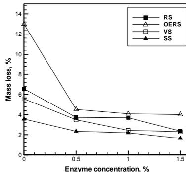
**Figure 4.** Mass loss values of samples related to enzyme concentrations after abrasion.
