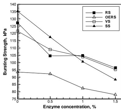
**Figure 5.** Bursting strengths of fabric samples versus enzyme concentrations.
