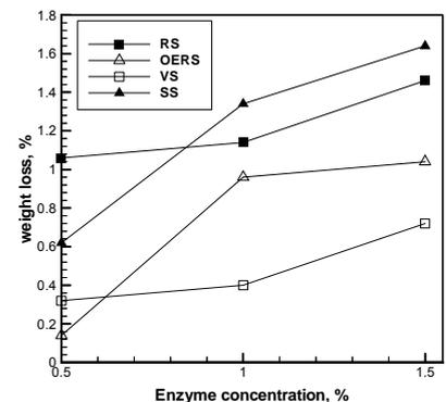
**Figure 4.** Weight loss (%) of fabric samples versus enzymatic concentration
