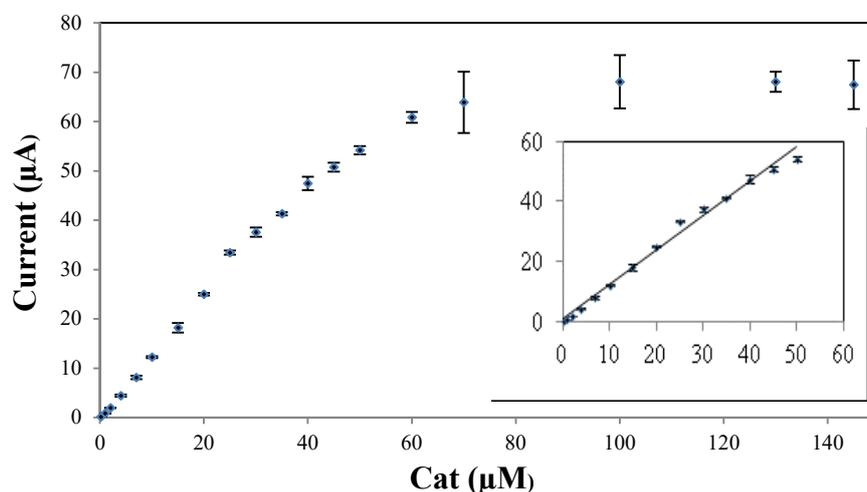
**Figure 6.** Calibration curve for Cat obtained Chit-GNP-T biosensor.
