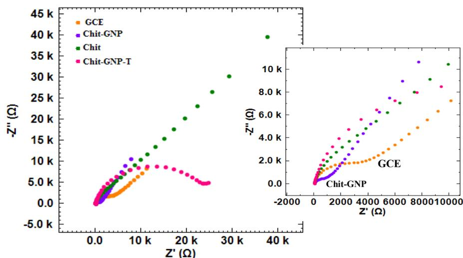
**Figure 1.** Nyquist diagram of GCE, Chit, Chit-GNP and Chit-GNP-T coated electrode in 0.5 mM  $K_4[Fe(CN)_6]$  containing 0.5 M  $KNO_3$  solution. Frequency range:  $10^5$ -0.1 Hz, amplitude: 0,005 V.
