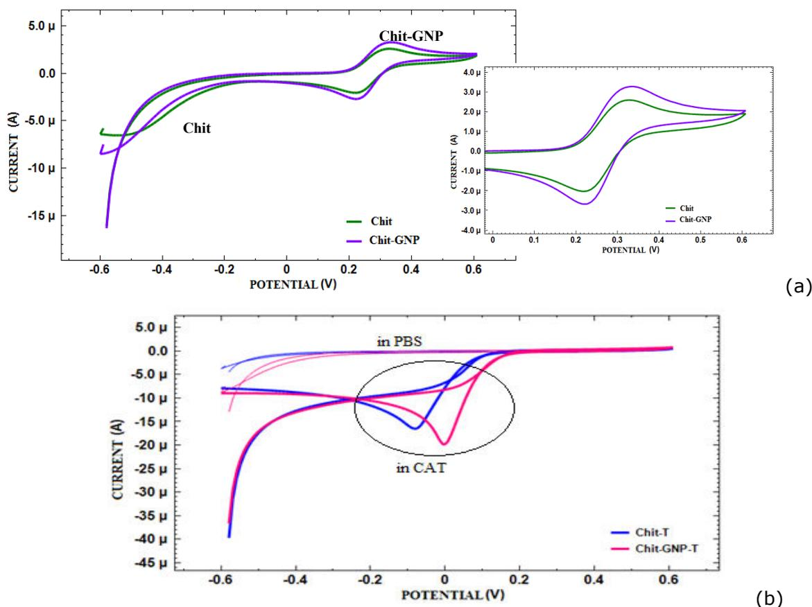
**Figure 3.** Cyclic voltammetry of Chit and Chit-GNP coated electrodes. Potential range:  $\pm 0.6$  V, scan rate: 0.01 V/s. (a) in 0.5 mM  $K_4[Fe(CN)_6]$  containing 0.5 M  $KNO_3$  solution. (b) in the absence and presence of 0.1 mM Cat containing PBS solution.
