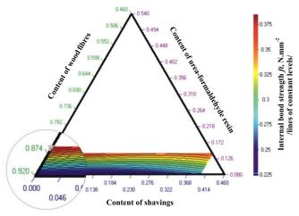
Fig. 3 "Composition-property" diagram for the internal bond strength of the combined fibreboards manufactured with coniferous wood shavings
