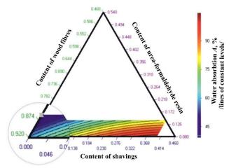
Fig.5 Composition-property" diagram for the water absorption of the combined fibreboards manufactured with coniferous wood shavings
