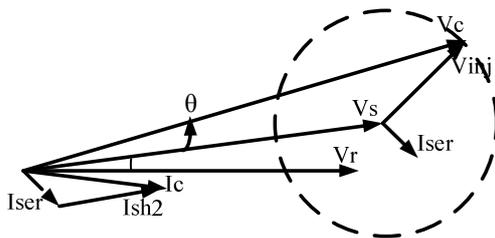
Figure 6. Phasor diagram of power system
