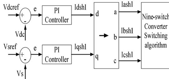
Figure 8. Circuit diagram to control DC link and sending end voltages
