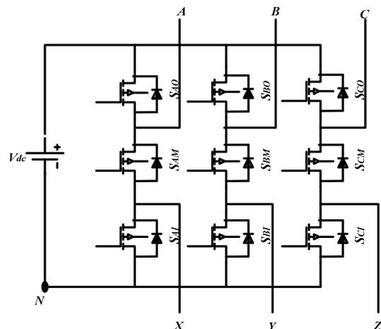
Figure 1. Structure of nine-switch ac/ac converter.
