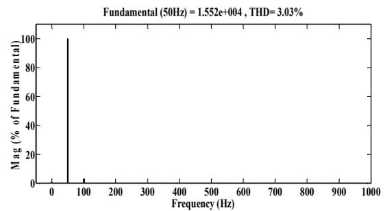
Figure 11. Harmonic spectrum of injected voltage
