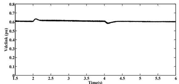
Figure 12. DC link voltage of nine switch converter
