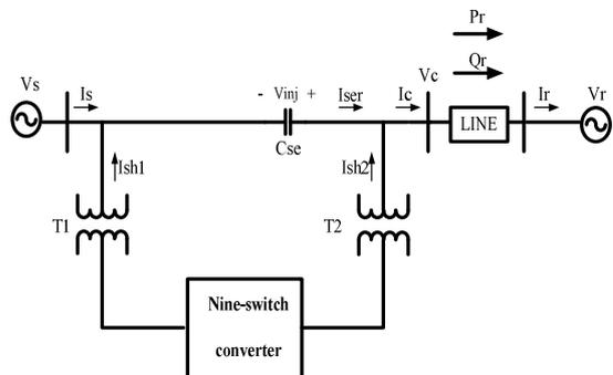
Figure 5. Proposed UPFC based on nine switch converter
