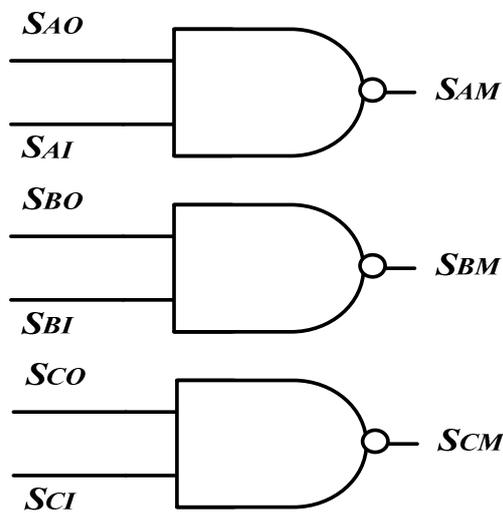
Figure 3. Circuit to generate middle switches gate signals.
