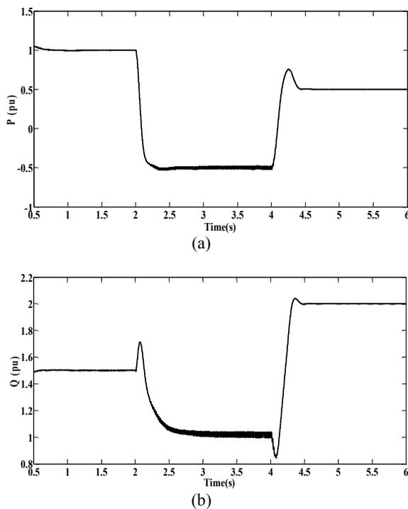
Figure 9. Receiving powers: (a) active power (b) reactive power
