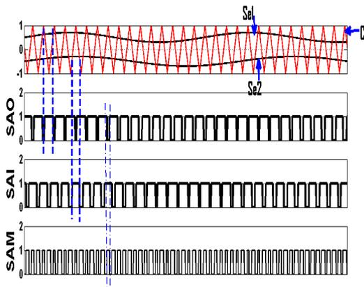
Figure 2. PWM waveforms for nine switch converter.
