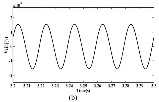
Figure 10. Injected series voltage by capacitor: a) during all simulation time, b) during short time to show sinusoidal series voltage.
