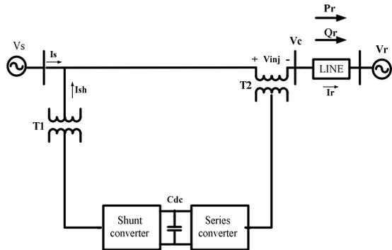
Figure 4. Conventional UPFC consist of shunt and series converters
