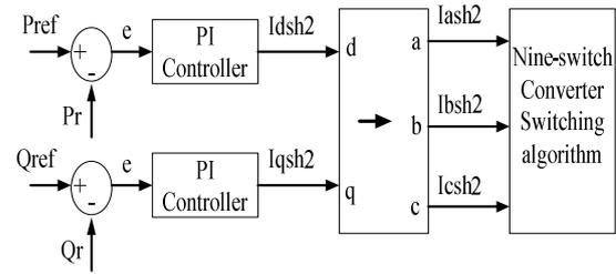
Figure 7. Circuit diagram to control active and reactive power
