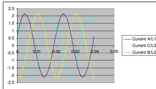
Figure 11. Stator current waveforms for the blocked rotor operation
