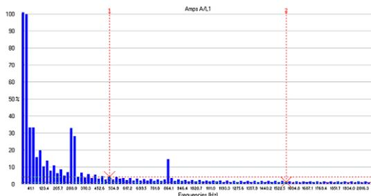
**Figure 6.** Harmonic spectrum of the rotor current waveform for no-load operation
