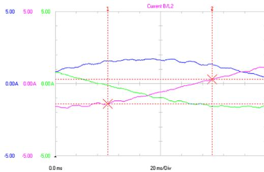
Figure 9. The rotor current waveform for load operation
