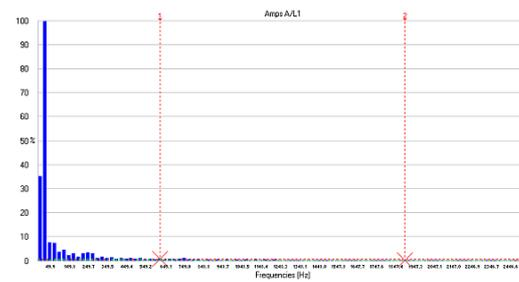
Figure 10. Harmonic spectrum of the rotor current waveform for load operation
