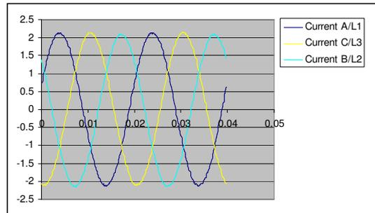
**Figure 3.** Stator current waveforms for no-load operation
