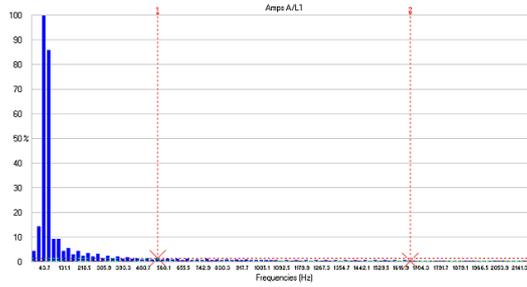
Figure 8. Harmonic spectrum of the stator current waveform for load operation
