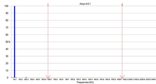
**Figure 12.** Harmonic spectrum of the stator current waveform for the blocked rotor operation
