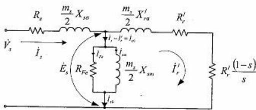
**Figure 2.** Equivalent circuit diagram for induction motor on a per phase basis referred to the stator.
