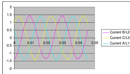
**Figure 7.** Stator current waveforms for load operation
