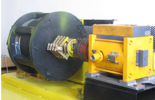
**Figure 1.** Inverted rotor induction motor
