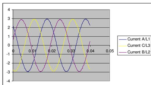
**Figure 13.** Rotor current waveforms for the blocked rotor operation
