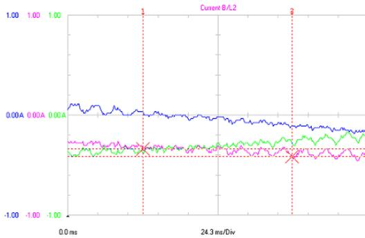
**Figure 5.** The rotor current waveform for no-load operation
