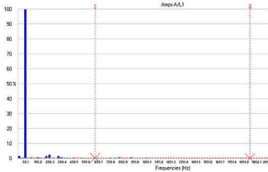
**Figure 4.** Harmonic spectrum of the stator current waveform for no-load operation
