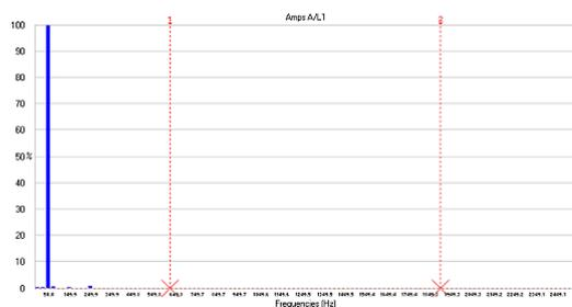
**Figure 14.** Harmonic spectrum of the rotor current waveform for the blocked rotor operation
