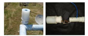
Figure 6. Assembly of the pyranometer beside a photodiode sensor (Campbell Scientific Inc., model LI200X) for comparison of the signals.
