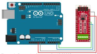
*Figure 4. Connection between the ADS1115x converter and Arduino UNO board.*
