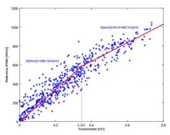
Figure 7. Cloud points used for calibration of the pyranometer.
