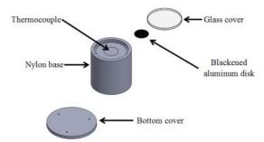
Figure 2. Exploded perspective of the pyranometer.
