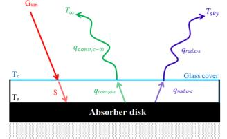
Figure 1. Schematic drawing of the thermal sensor depicting the energy conservation on the absorber disk.
