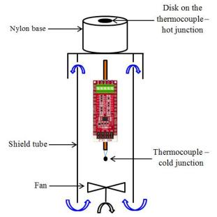
Figure 5. Pyranometer assembly with cooling system.
