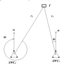
**Fig. 5.** The determination of the target location by triangulation:  $r_1$  and  $r_2$  are distances to target *T*;  $\alpha$  is a reference direction;  $\varphi_1$  and  $\varphi_2$  are directional angles.
