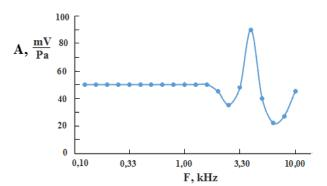
Fig. 2. Acoustoelectric characteristics of the piezoelectric detector.
