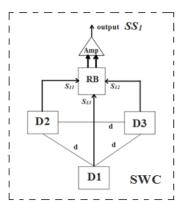
**Fig. 4.** The chart of the Seismic Waves Cell (SWC). D1, D2, D3 – 3D seismic detectors; RB - receiving box; Amp – amplifier; d – distance between detectors (base of SWC).
