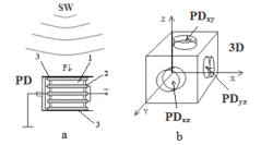
**Fig. 3.** Design of a single-dimensional PD (a) and 3Ddimensional (b) piezoelectric detectors: 1–piezoelectric plates; 2–foil layers, 3– insulating layers;  $PD_{XY}$ ,  $PD_{XZ}$  and  $PD_{YZ}$  are piezoelements allocated on the *XY*, *XZ*, and *YZ* planes, correspondingly; SW- seismic wave.
