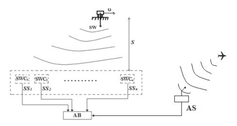
**Fig. 6.** Seismic location station SLS. SWC<sub>i</sub> - seismic waves cells;  $SS_i$  – output signals from SW<sub>i</sub>; SW – seismic waves from moving truck; v - velocity of truck; S – distance to moving truck-target; AB - analyzing block; AS-acoustic system.
