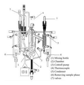
Figure 1. Fisher ebulliometer model 602.
