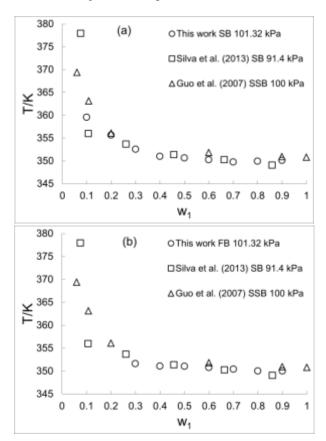
Figure 3. Agreement of VLE data for systems (a) ethanol + soybean oil biodiesel (SB) and (b) ethanol + frying oil biodiesel (FB) with boiling points reported [11],[15].
