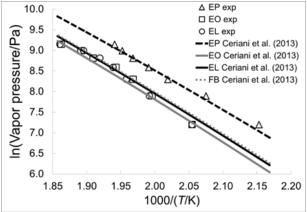
Figure 4. Experimental [28-32] and predicted vapor pressure for (a) methyl esters and soybean oil biodiesel adopted; (b) ethyl esters and frying oil biodiesel adopted.
