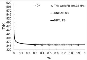
Figure 5. Experimental and calculated bubble-point temperature data using UNIFAC and NRTL models for systems (a) ethanol + SB and (b) ethanol + FB.
