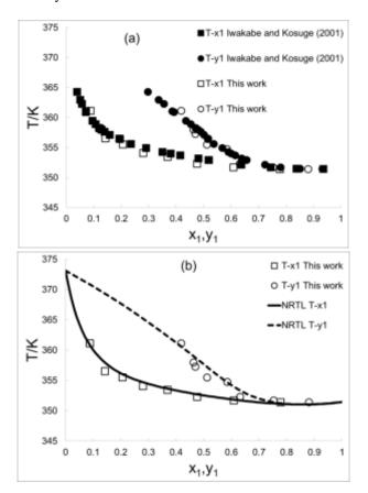
Figure 2. Comparison of VLE data measured for ethanol + water system at 101.32 kPa (a) with reported data [24] at same pressure and (b) with VLE obtained by NRTL model.
