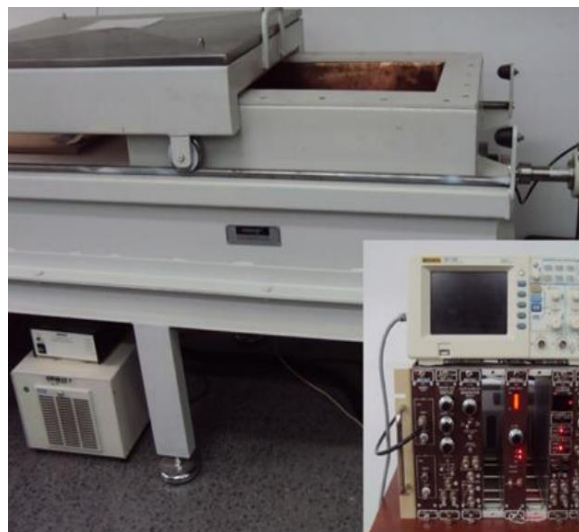
Figure 2. The HPGe detector system used in our studies.
