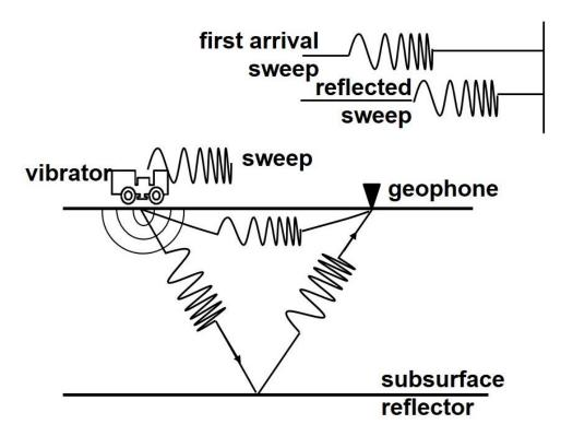
Figure 1b. Schematic view of vibroseismic technique (revised from Crawford et al., 1960; Seriff and Kim, 1970; Chapman et al., 1981 and Pann, 1986).
