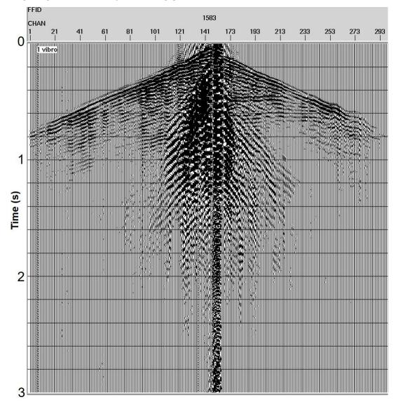
Figure 6c. 2D shot gather with 1 vibrator (Parameters are *12-64 Hz, 4 sweeps, 12 sec., Non-Linear -3 dB/Oct., Drive level 80%*).
