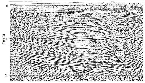
Figure 8b. Example of seismic section with 6 sweeps line-B (Parameters are 10-72 Hz, 8 sec., Linear, Drive level c=37%, 4 vibrators).
