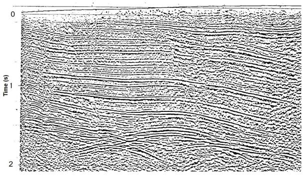
Figure 8a. Example of seismic section with 4 sweeps line-A (Parameters are 10-72 Hz, 8 sec., Linear, Drive level c= 80%, 4 vibrators).
