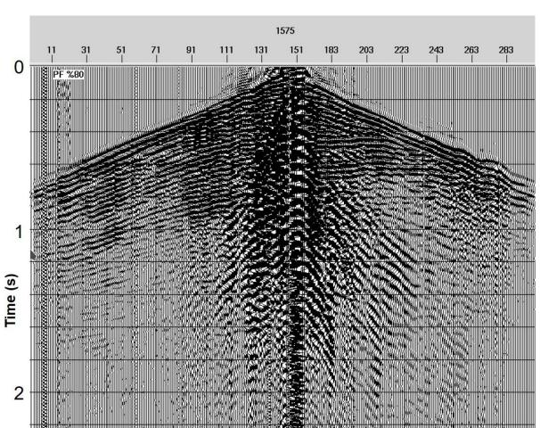
Figure 5d. 3D shot gather with *80%* peak-force (Parameters are 12-64 Hz, 4 sweeps, 12 sec, Non-Linear -3 dB/Oct., 4 vibrators).
