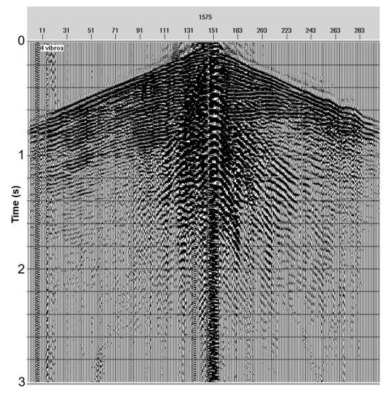
Figure 6d. 2D shot gather with 4 vibrator (Parameters are 12-64 Hz, 4 sweeps, 12 sec., Non-Linear -3 dB/Oct., Drive level 80%).
