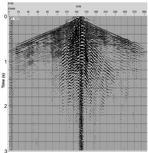
Figure 5c. 2D shot gather with 37% peak-force (Parameters are 12-64 Hz, 4 sweeps, 12 sec, Non-Linear -3 dB/Oct., 4 vibrators).
