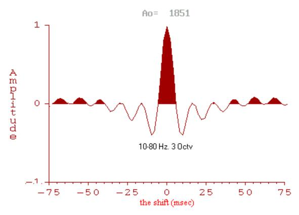
Figure 2d. Autocorrelation of sweep. *Şekil 2d. Sweep'in otokorelasyonu.*
