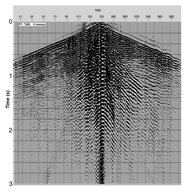
Figure 10b. 2D shot gather with Drive level 80% (High force) and 4 sweeps (Parameters are 12-64 *Hz, 12 sec., Non-Linear -3 dB/Oct., 4 vibrators*).
