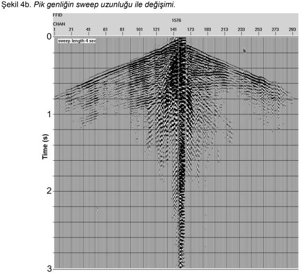
Figure 4c. 2D shot gather with 4 sec sweep length (Parameters are 12-64 Hz, 4 sweeps, Non-Linear -3 dB/Oct., Drive level *80%*, 4 vibrators).
