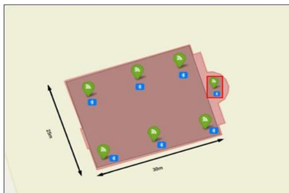
Figure 7. The Warehouse and The Placed Beacons
