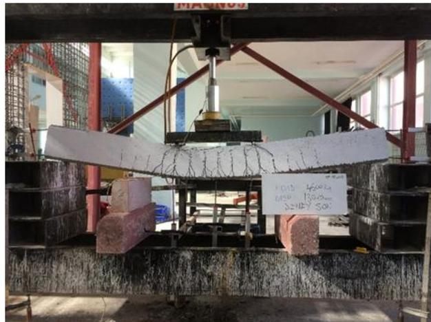
**Figure 11.** Fractures in specimen (B-7)
