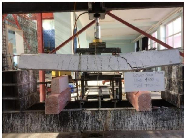
**Figure 4.** Fractures in specimen (B-1)
