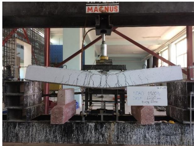
Figure 13. Fractures in specimen (B-4)
