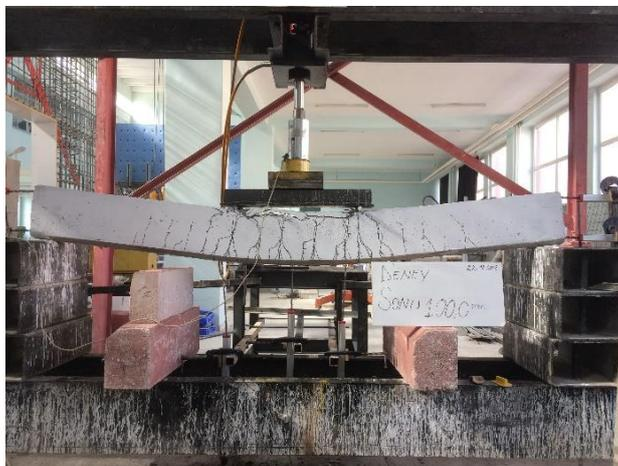
Figure 14. Fractures in specimen (B-8)
