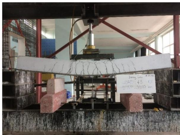
**Figure 5.** Fractures in specimen (B-5)
