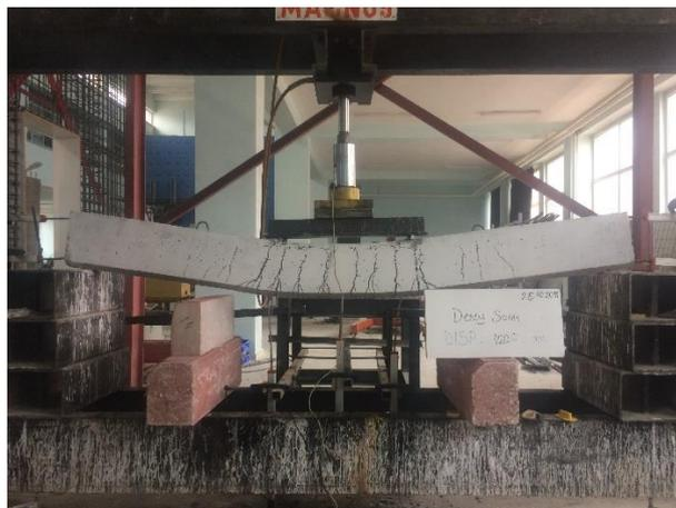
**Figure 8.** Fractures in specimen (B-6)
