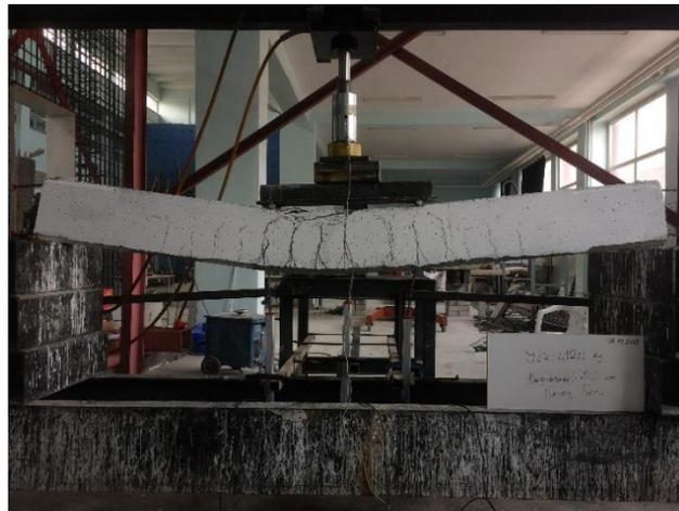
**Figure 10.** Fractures in specimen (B-3)
