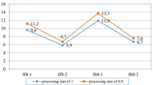
Figure 4. Manufacturing lead times for 8-workstation systems with various layouts in the cases of processing rates of 1 and 0.9 per unit time (cases 4, 5, 6 & 7 vs. 12, 13, 14 & 15)
