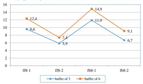
*Figure 3.* Manufacturing lead times for 8-workstation systems with various layouts in the cases of buffer sizes of 3 and 6 (cases 4, 5, 6 & 7 vs. 8, 9, 10 & 11)
