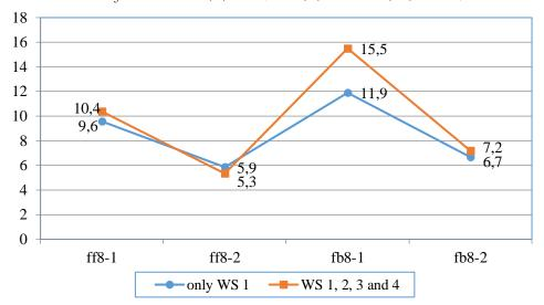
*Figure 5. Manufacturing lead times for 8-workstation systems with various layouts in which entry workstations are only WS 1 and WS 1, 2, 3 & 4 (cases 4, 5, 6 & 7 vs. 16, 17, 18 & 19)*
