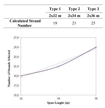
Figure 12. Span Lengths vs. Strands Graph
