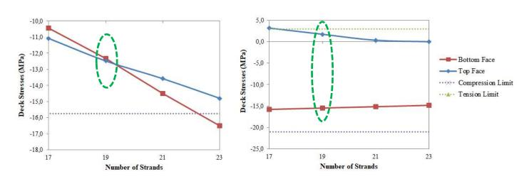
Figure 9. Deck Type 1, Stresses vs. Strands Graph (First Stage & Service Stage, Respectively)
