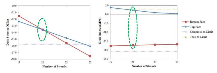
Figure 10. Deck Type 2, Stresses vs. Strands Graph (First Stage & Service Stage, Respectively)
