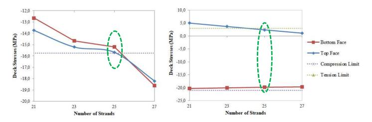
Figure 11. Deck Type 3, Stresses vs. Strands Graph (First Stage & Service Stage, Respectively)
