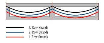
Figure 6. Strands Longitudinal Section Layout
