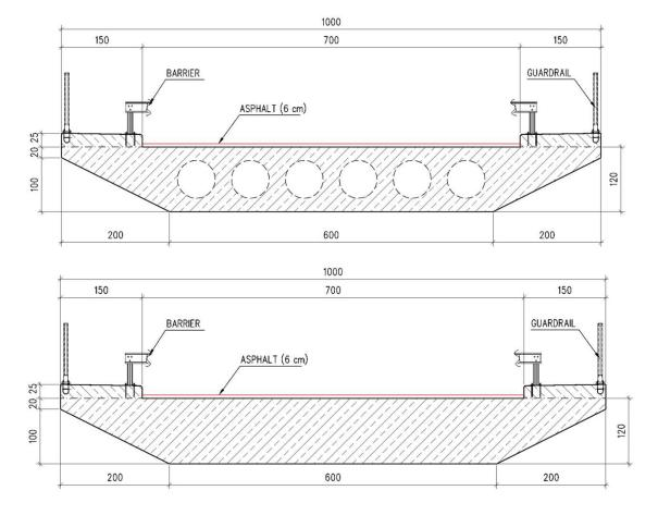
Figure 1. Voided and Filled Deck Typical Sections
