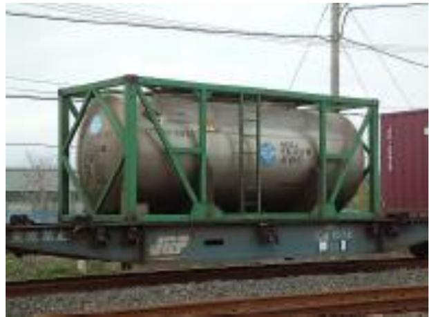
Fig. 2: A standard freight tank container,(Chatama [GFDL (URL 1) or CC BY-SA 3.0 (URL 2).
