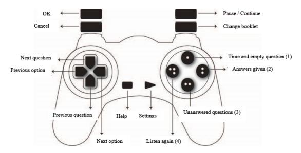
Figure 1. Schematic representation of the remote and the functions of the keys
