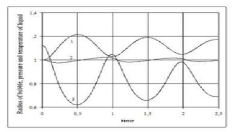
Fig. 2: Dependences of the radius of the bubble, pressure and air temperature in the bubble on time at pressure decrease in liquid
