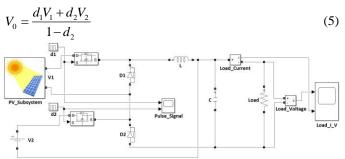
Fig. 4. Two-input single-output buck / buck-boost converter circuit
