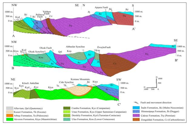
Figure 13- Geological cross-sections showing the imbricated structure of the study area (Sunal and Tüysüz (2002), see the geology map in Figure 2 for section locations).
