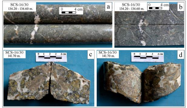
Figure 14- The disseminated galena+sphalerite+chalcopyrite-bearing barite+quartz+calcite veins-veinlets determined in the drilling studies in altered andesites; a), b) disseminated galena+sphalerite+chalcopyrite mineralization in barite+quartz+calcite+dolomite veins, c), d) densely disseminated galena+sphalerite+chalcopyrite mineralization within barite+quartz+calcite+dolomite vein-veinlets.
