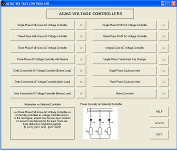
Figure 1. The main window of the GUI (Şekil 1. GUI ana penceresi)
