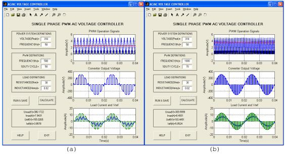
Figure 3. The individual window of single-phase pwm ac voltage controller for different pwm operations, a) f=500Hz - DCycle=%50, b) f=1000Hz - DCycle=%70
