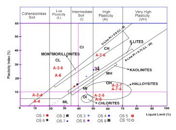
Fig. 8. Casagrande Plasticity Chart for the sampled soils showing predominantly High Plasticity
