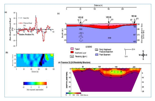
Fig. 12. (a) VLF-EM Real and Filtered Real Components, (b) VLF-EM 2-D Model, (c) Geoelectric Section, (d) Dipole-Dipole Resistivity Structure along Traverse 32 (Ifon-Ose)
