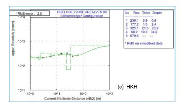
Fig. 10. Typical Curve Types obtained in the study area
