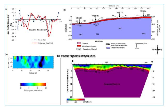
Fig. 11. (a) VLF-EM Real and Filtered Real Components, (b) VLF-EM 2-D Model, (c) Geoelectric Section, (d) Dipole-Dipole Resistivity Structure along Traverse 29 (Ido Ani-Ose)
