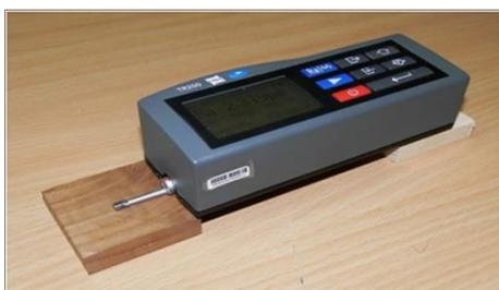
**Figure 4.** Stylus contact tester (TR200 TIME, China) for measurement of parameter Ra
