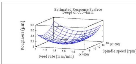
**Figure 6.** Surface roughness Ra response surface graph for treated wood at 160°C and raster processing strategy
