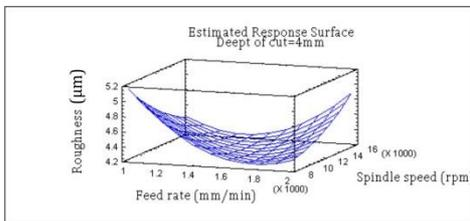
**Figure 5.** Surface roughness Ra response surface graph for untreated wood and raster processing strategy
