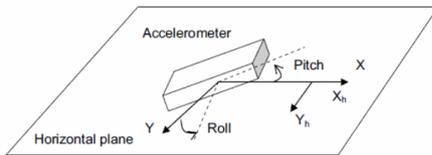
Figure 3. IMU at tilted position.
