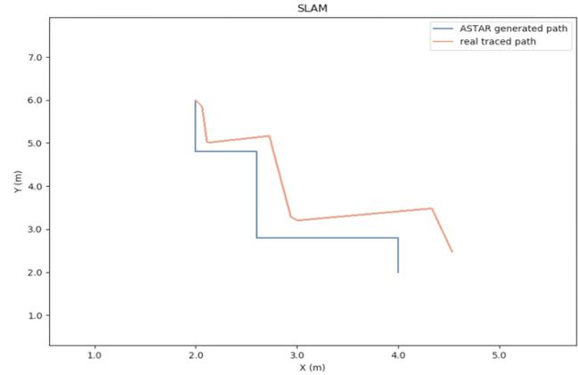
**Figure 11.** Performance for a zig-zag trajectory (with sensor fusion).
