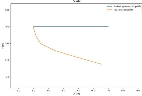
**Figure 9.** Performance for a straight trajectory (without sensor fusion).
