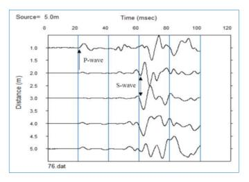
Fig. 3a. Typical seismic record 15-m depth
