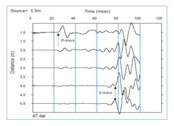
Fig. 3b. Typical seismic record 20-m depth
