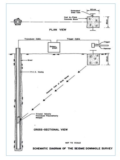
Fig. 2. Schematic diagram for downhole seismic survey
