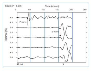
Fig. 3d. Seismic record 20-m depth
