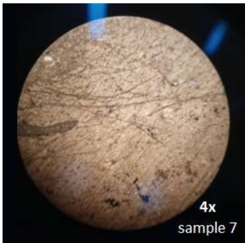
Fig. 6. Microfractures and organic matter
