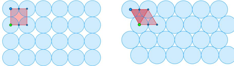
Figure 1. Comparison of the gaps between circles in the quadratic and hexagonal packing models of 24 isodiametric circles.
