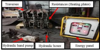
Figure 6. Vulcanization system equipment
