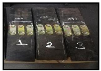
Figure 9. Image of belt specimens with mechanical splicing
