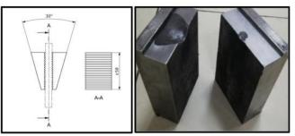
Figure 11. Technical drawing and image of the holding jaws
