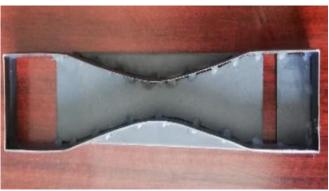
Figure 1. Image of bow tie specimen apparatus according to ISO 37 Standard [13]
