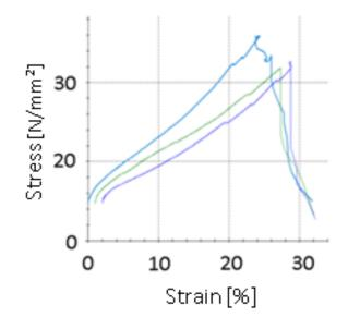
Figure 15. Tensile testing graphs of vulcanized bonded belt specimens
