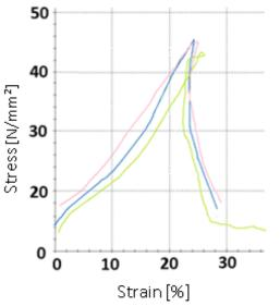
Figure 14. Tensile testing graph of unspliced belt specimens
