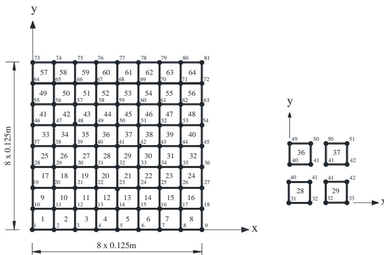
Figure 2. Finite element mesh of the plate
