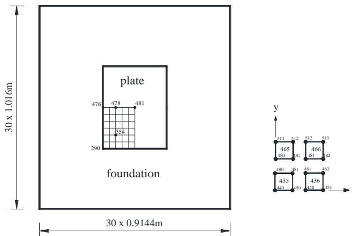
Figure 4. Finite element mesh of the plate-foundation system
