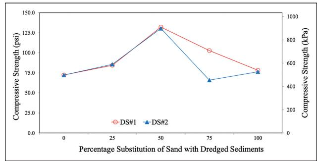
Figure 6. Variation of unconfined compressive strength with percentage substitution of sand with dredged material.
