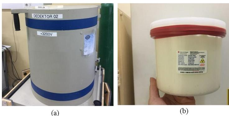
**Figure 1.** a) HPGe Detector, b) Marinelli beaker with 0.5 g/cc density used in the experiment
