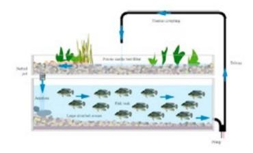
Figure 3: Basics of an Aquaponic System [17].
