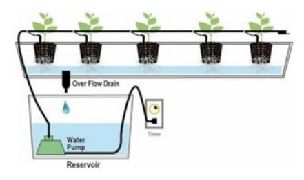
Figure 4: Basics of Aeroponic System [37].
