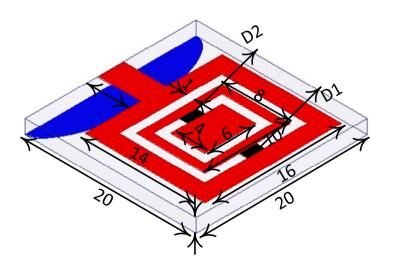
Fig.1 configuration of antenna structure
