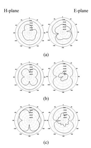
Fig. 3Simulated radiation patterns for the dual notch band performance of the proposed antenna at(a: 2.4 GHz, b: 4 GHz and c: 5.5 GHz)
