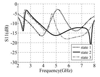
**Fig. 2.** Simulated S<sub>11</sub> of the proposed reconfigurable Multiband antenna for different biasing statuses of the PIN diodes in Table 1.
