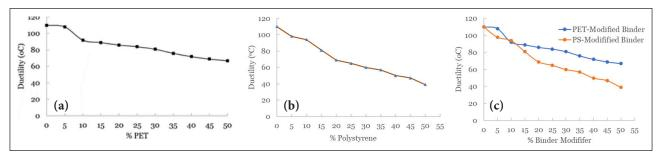
**Figure 6**. **(a)** Influence of PET on modified binder ductility **(b)** influence of PS on binder modified binder **(c)** Comparative ductility curve.
