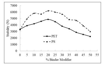
Figure 9. Stability of PET and PS modified asphalt.
