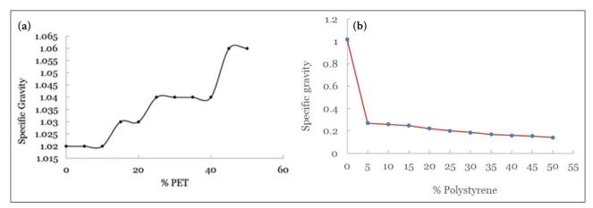
Figure 5. (a) Specific gravity of PET-Modified binder, (b) Specific gravity of PS-Modified binder.
