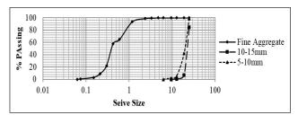
Figure 2. Particle Size Distribution curve of aggregate used.
