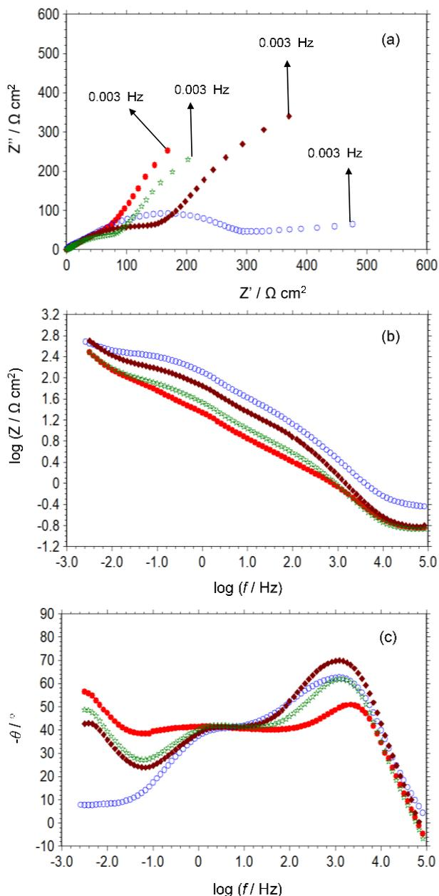
**Figure 2.** The Nyquist (a), log Z-log f (b), and phase angle-log f (c) (Bode) plots of Cu obtained in 1 M HCl solution without (●) and with the addition of 1000 ppm RRF (○), RRL (◆) and RRR (☆) solutions after 1-hour exposure
