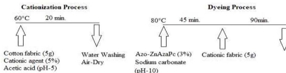
Figure 2. Cationization and dyeing process conditions.
