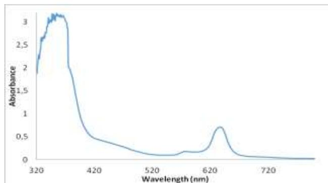
Figure 3. UV/Vis spectrum of AzaPc **1a**.
