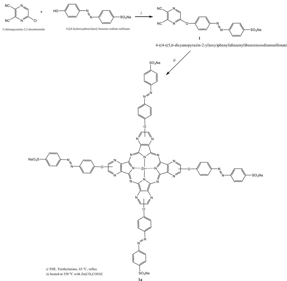
**Figure 1.** Synthesis of water soluble azaphthalocyanine containing azo groups.
