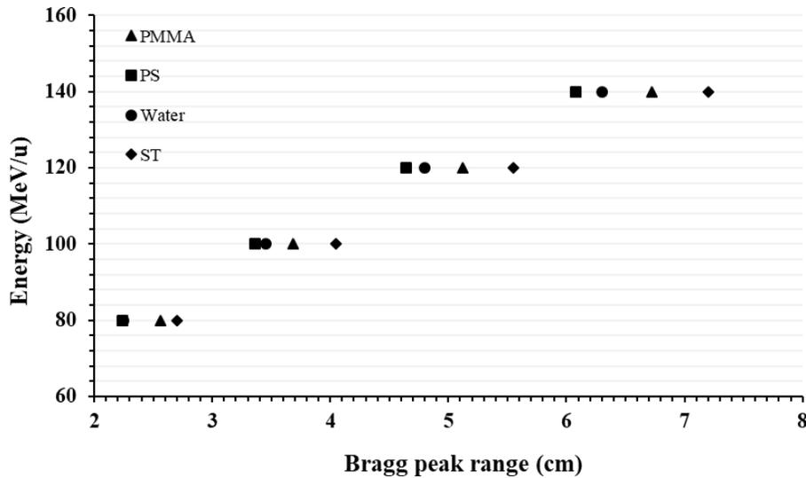
FIGURE 1. Bragg peak range (cm) created by the  $^{10}\text{B}$  ion beam in four phantoms.
