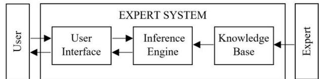
Figure 2. The general structure of expert systems [21]
