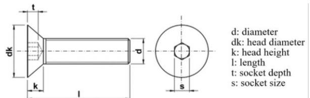
Figure 8. Countersunk bolt
