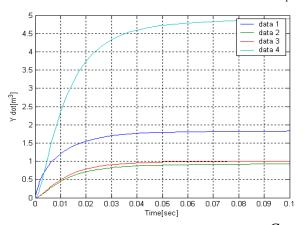
Fig 1.24: Effect of the Capacity of tank on the Process, with  $\,C_1^{}$  =3e-03
