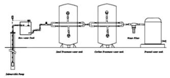
$\textbf{Fig 1.1.} \ \ \textbf{Flow sheet of a Simple water treatment plant}.$
