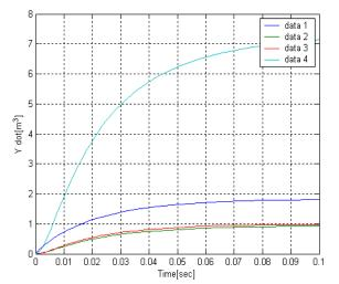
Fig 1.34. Effect of the Capacity of tank on the Process, with  $C_3$  =1300e-03
