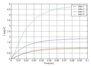
Fig 1.31. Effect of the Capacity of tank on the Process, with  $C_2$  =7e-03
