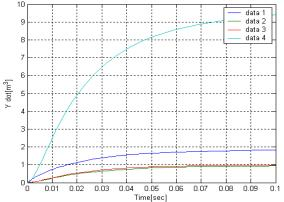
Fig 1.33. Effect of the Capacity of tank on the Process, with  $\,C_3 = 1000 \mathrm{e}^{-03}$
