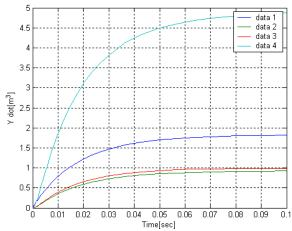
Fig 1.29. Effect of the Capacity of tank on the Process, with  $C_2$  =3e-03
