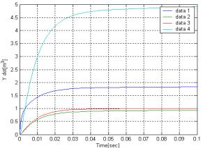
Fig 1.23. Effect of the Capacity of tank on the Process, with  $C_1$  =1e-03
