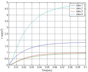
Fig 1.16. Effect of Restriction to flow on the Process, with  $R_3 = 7.0$
