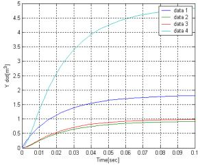
Fig 1.37. Effect of the Capacity of tank on the Process, with  $C_3$  =1900e-03
