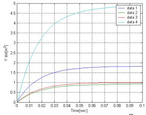
Fig 1.28. Effect of the Capacity of tank on the Process, with  $C_2$  =1e-03
