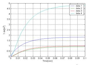
Fig 1.26: Effect of the Capacity of tank on the Process, with  $\,C_1$  =7e-03
