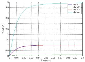
Fig 1.8. Effect of Restriction to flow on the Process, with  $R_2$  =0.1
