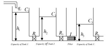
Figure 1.2. Coupled tank flow System.
