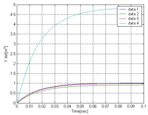
Fig 1.3. Effect of Restriction to flow on the Process, with  $R_1 = 0.1$
