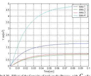
Fig 1.30. Effect of the Capacity of tank on the Process, with  $C_2$  =5e-03
