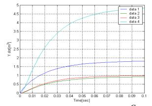
Fig 1.32. Effect of the Capacity of tank on the Process, with  $C_2$  =9e-03
