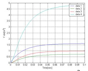
**Fig 1.11.** Effect of Restriction to flow on the Process, with  $R_2 = 0.7$
