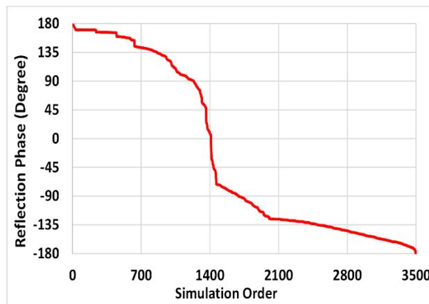
**Figure 10.** Phase response plot for Circle-Minkowski reflective unit cell (With Rotation)
