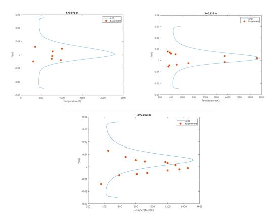
Figure 3. Comparison of experimental and analysis results for x=0.078m, x=0.125m and x=0.233m
