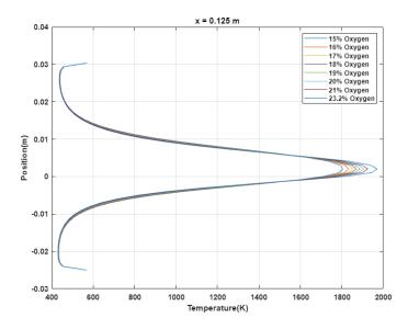
Figure 5. Temperature graphs for x=0.125 m
