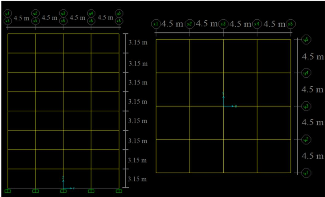
**Figure 1.** The dimensions of the steel structure model
