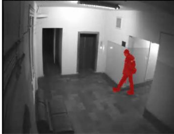
**Figure 2:** Simple background modeling motion detection [13]
