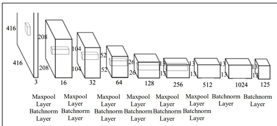
**Figure 3:** Tiny YOLOv2 Architecture [22]
