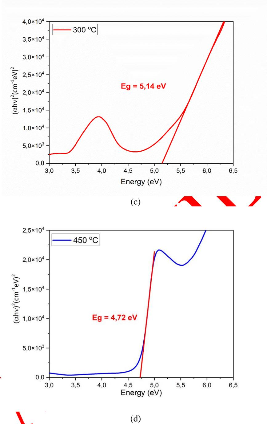
**Figure 5.** Absorption spectrum and  $(\alpha hv)^2$  vs  $hv$  plots for Graphene Oxide thin films deposited on p-Si substrate at 8 mTorr pressure and (b) 150 °C, (c) 300 °C, (d) 450 °C temperatures
