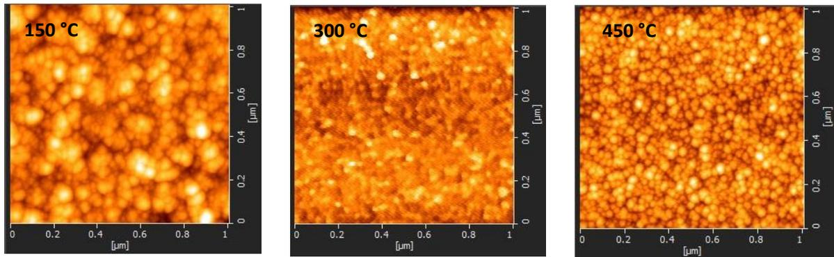
**Figure 4.** AFM views of  $Ga_2O_3$  thin films prepared at 150 °C, 300 °C, 450 °C substrate temperatures
