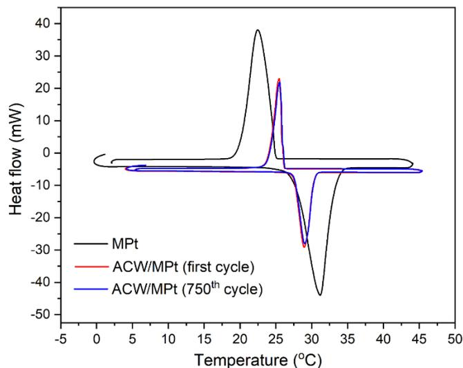
Figure 4. DSC thermograms of MPt and ACW/MPt
