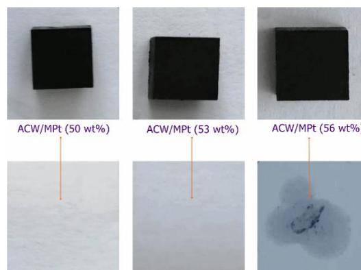
Figure 1. The leakage test result of ACW/MPt samples
