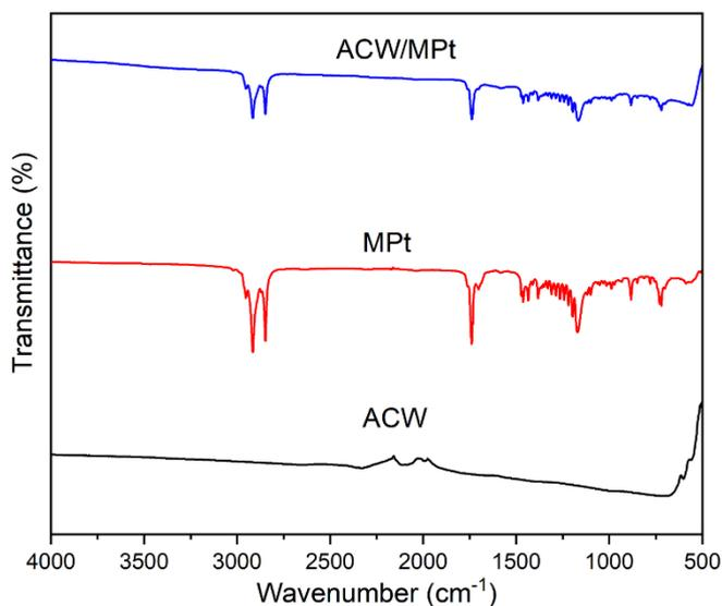
Figure 3. FTIR spectra of MPt, ACW and ACW/MPt
