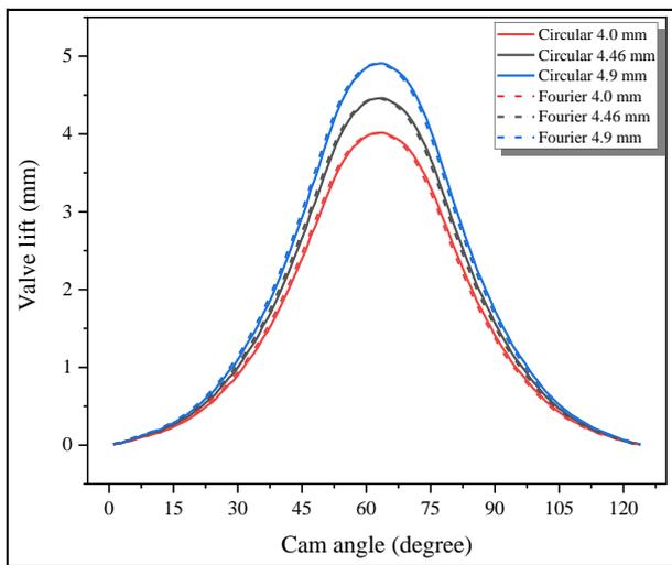
Fig. 3. Valve lift of the cams designed with the circular arc curve method and extrapolated with the Fourier series.
