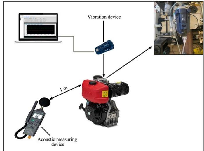
Fig. 1. The schematic representation of the experimental study.
