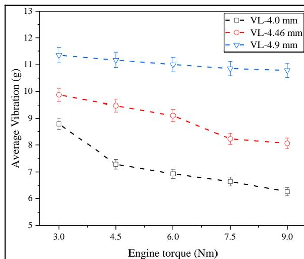
Fig. 10. The effect of valve lift variation on average vibration under different engine load conditions.
