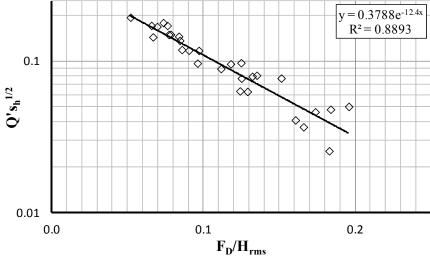
Figure 5. Variation of dimensionless discharge with disturbed freeboard.
