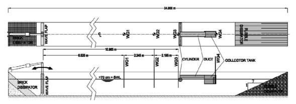
Figure 1. Plan and profile view of the wave flume.
