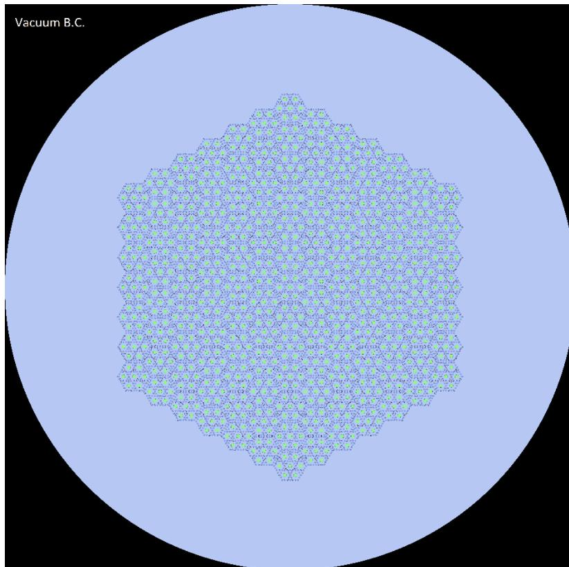
**Fig. 2.** Horizontal Section of the HTGR full core model
