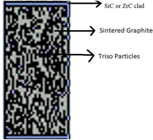
**Fig. 4.** Calculation fuel pellets model of fuel assembly
