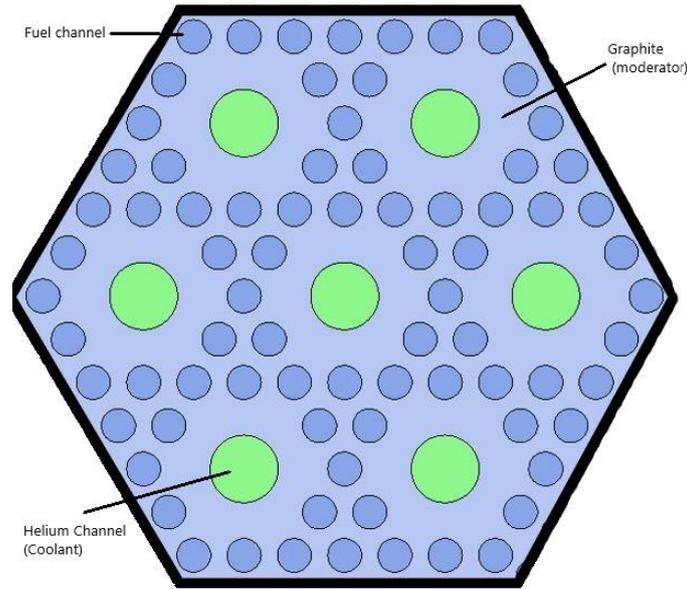
**Fig. 3.** Hexagonal bundle assembly view of the HTGR
