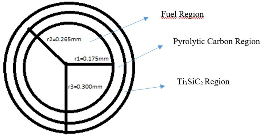
**Fig. 5.** TRISO particles of the fuel pellets model of fuel assembly
