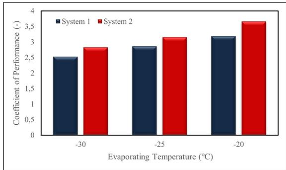
**Figure 4.** The COP values according to evaporator temperatures
