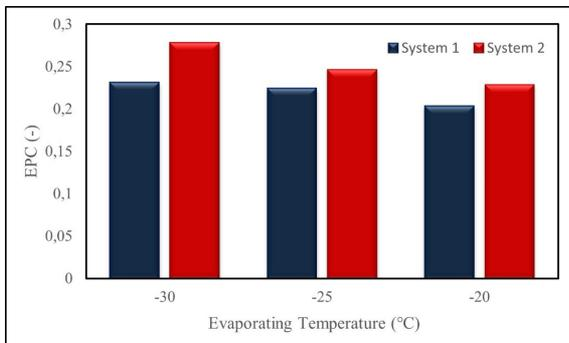
**Figure 6.** The EPC values according to evaporator temperatures
